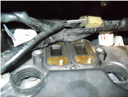
**STEP 9:** Remove the internal flange plates and unscrew the two bolts (photo). This will let you remove the screws and the metallic clamps that are attached on the plates. Then reinstall the flange plates on the engine cover.
