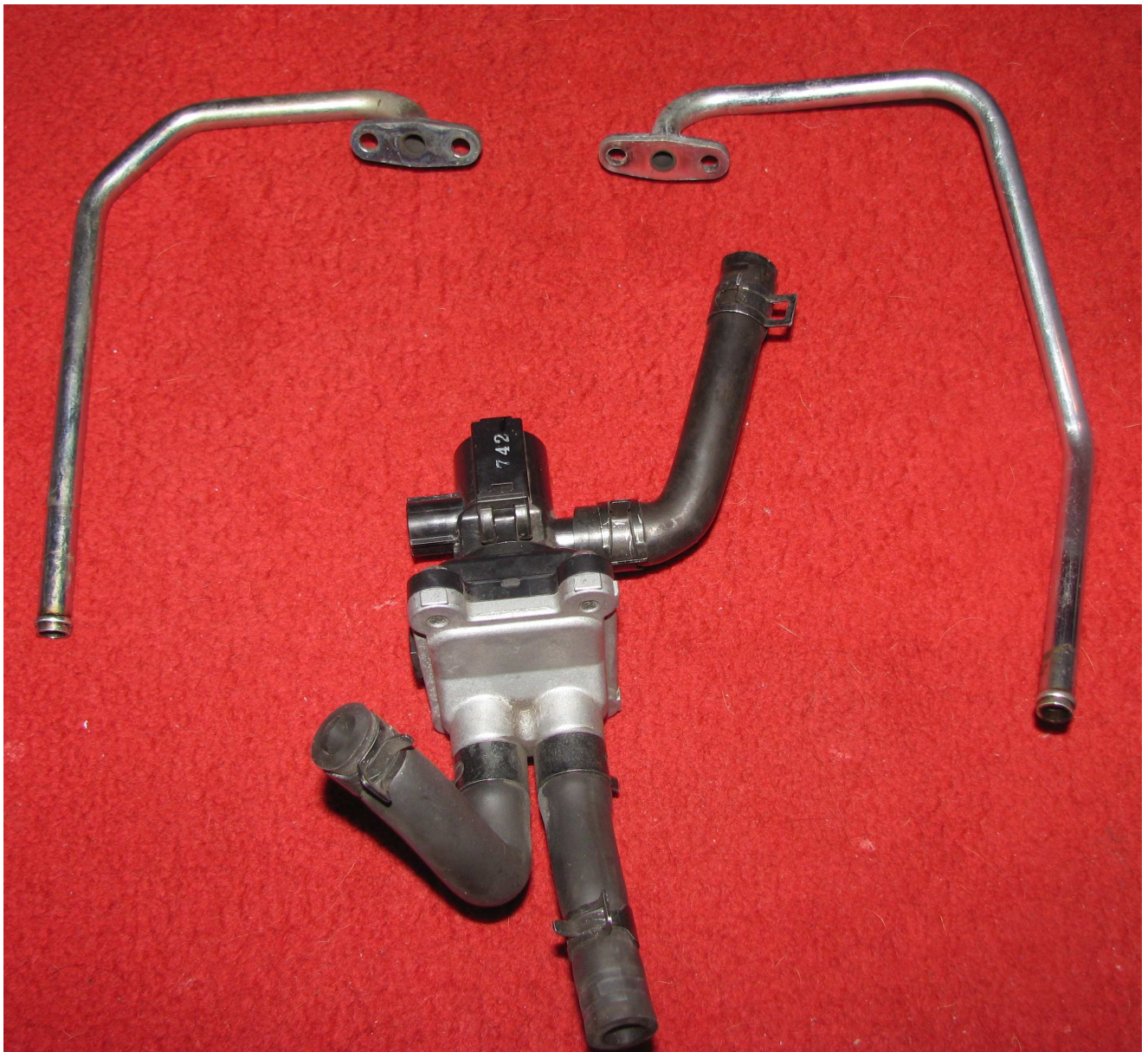
View of the dismantled parts - air pump and two pipes from the cylinders.
