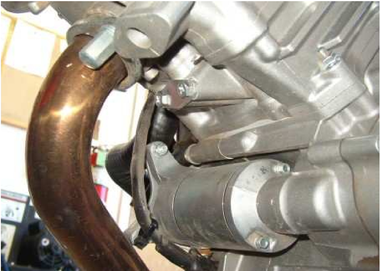
View blocked the AIS on the front cylinder (the view from the left)
