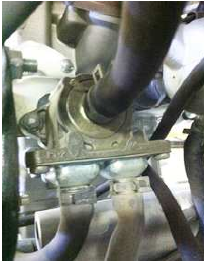
View of the air pump with cables - two lower steel tubes going to the cylinders and the upper to the airbox.
