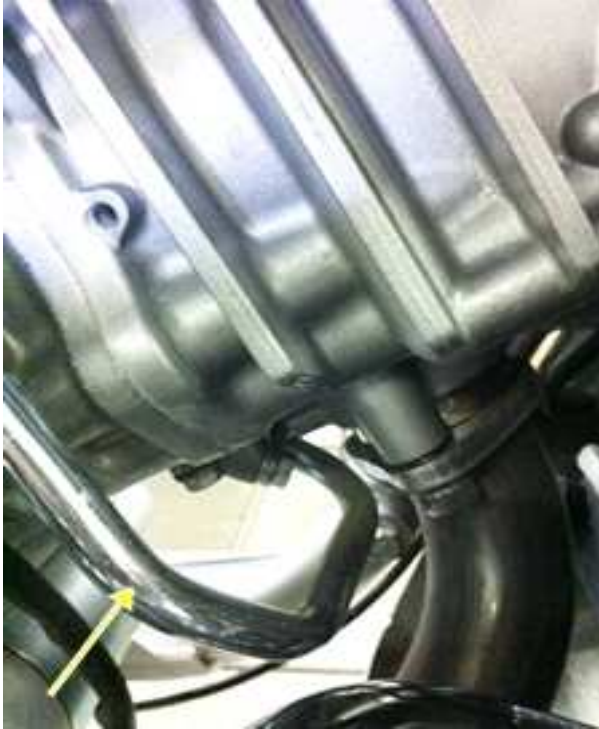
The arrangement of the AIS - the tube around the front and rear of the cylinder to be removed.
