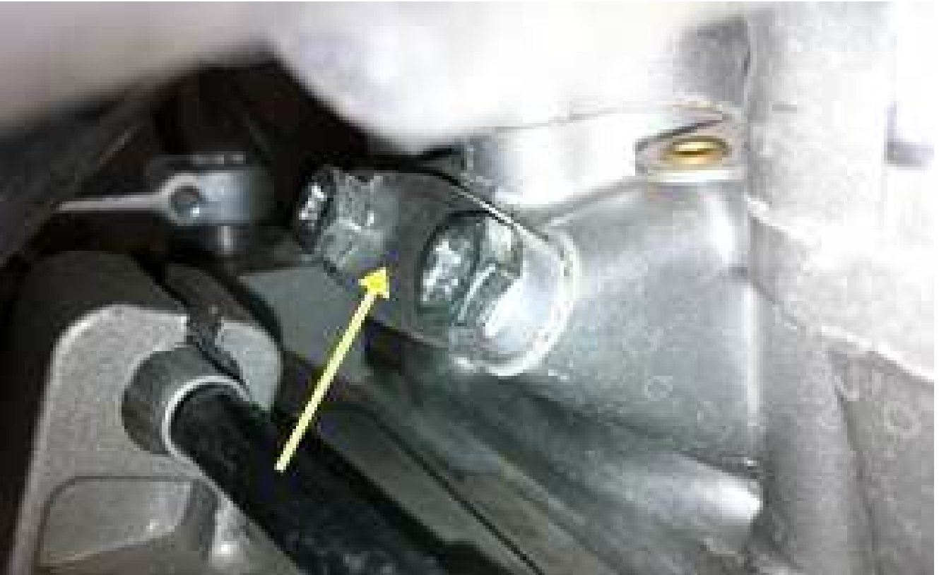
AIS slot sealed rear cylinder (viewed from the right) after removal of the tube blinds aluminum profile with a washer on the two screws.
