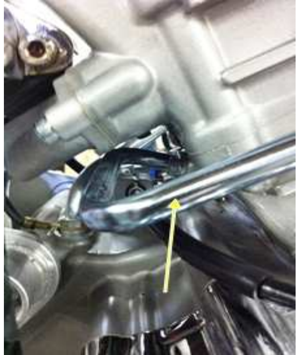
The arrangement of the AIS - the tube around the front and rear of the cylinder to be removed.
