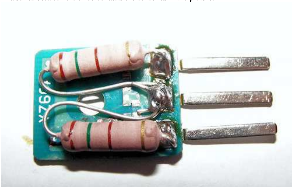
View of resistors soldered to the contact sensor
