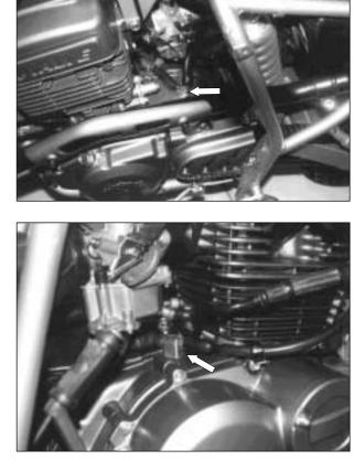
• Disconnect the lead wire of starter motor.
