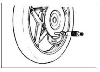
• With the disc mounted on the wheel check the disc for face runout with a dial gauge, as shown.
