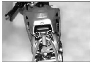
$\bullet$  Disconnect the  $\ominus$  and  $\oplus$  lead wires of battery (1).
