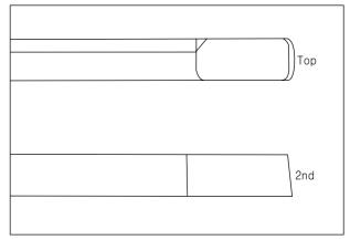
Install expander ring into the 2nd ring groove. Top and 2nd rings have the letter "R" or "Y" marked on the top. Be sure to bring the marked side to the top when fitting them to the piston.
