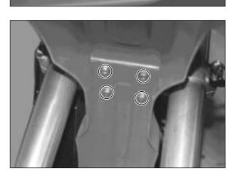
• Remove the handlebars clamp bolts.
