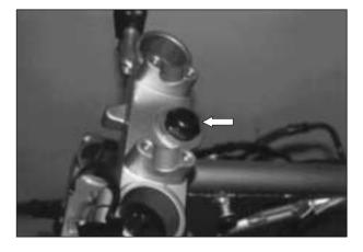
• Remove the steering stem nut and draw out the steering stem.
