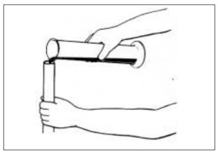
• Hold the front fork vertical and adjust the fork oil level with the special too.
