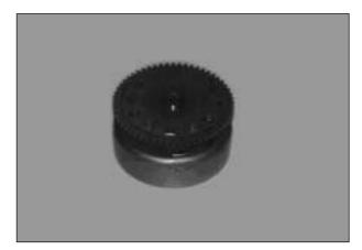
• Tighten the magneto rotor nut to the specified torque.
