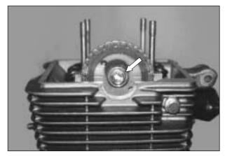
Remove the camshaft ①, cam sprocket ② and C-ring ③
