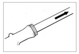
Remove the snap ring by using the special tool.
