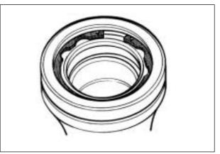
• Remove the oil seal by using the special tool.
