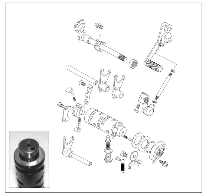
• Fit the gear shifting cam on the crankcase. Position the cam as shown in Fig. So that the gear shifting fork can be installed easily.
