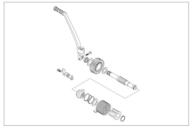
• When fitting the kick starter to the shaft, be sure to align the punched marks..
