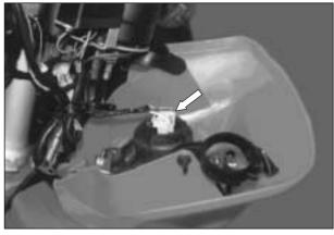
• Remove the two screws of the headlight housing.
