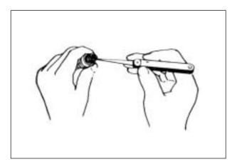
• Check the gap with a thickness gauge.
