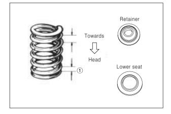
• Fit valve spring retainer, compress spring with a valve spring compressor and insert cotters.
