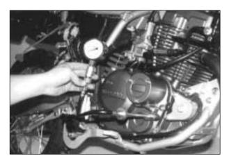
It the oil pressure is lower or higher than the specifications, several causes may be considered.
