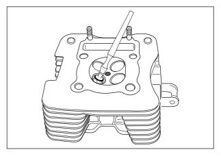
• The ring-like dye impression left on the valve face must be continuous-without any break. In addition, the width of the dye ring, which is the visualized seat "width", must be within the specification.
