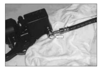
• Remove the two clamp bolts and take off the master cylinder.
