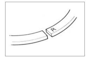
Position the gaps of the three rings as shown. Before inserting piston into the cylinder, check that the gaps are so located.
