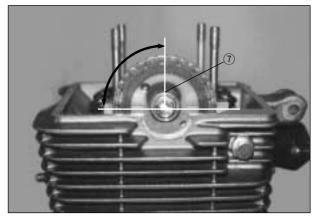
• Install the camshaft lock C-ring ①.
