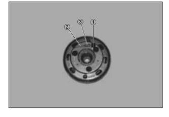
Clamp the rotor with a vise taking care not to damage it and remove the three bolts using the 5 mm "T" type hexagon wrench.
