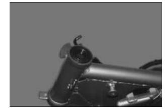
• Remove the upper and lower bearing.
